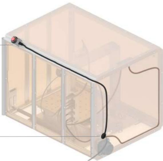
**05/06** Insert the other end of the long cable into either of the Expansion Ports of the Enclosure Converter.
